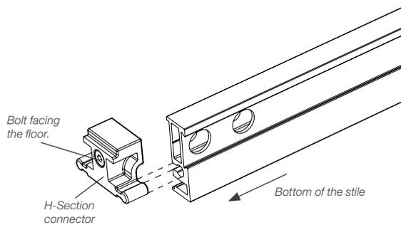
**A** Slide the H-Section connector into the matching hole in the stile.
