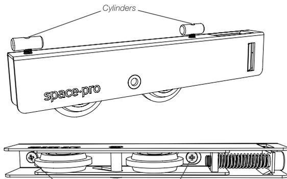
**A** Loosen the screws in the wheel to allow the cylinder to slide freely into the bottom rail.
